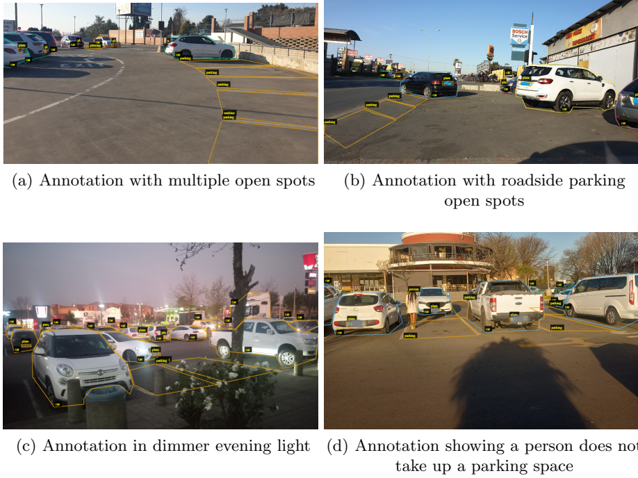
Fig. 1: The sample images above show the different scenarios that may be encountered in parking lots, and how the the annotations will look like to the Detectron2 model.
